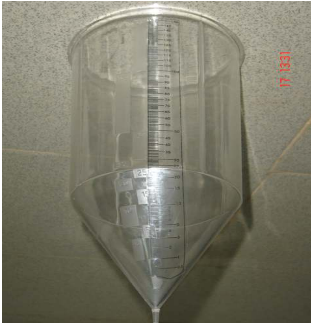
SIMPLIFIED LOCALLY MANUFACTURED RAINGAGE
